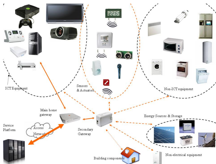
Figure 2: Perimeter of a home area network extended to a « Smart Home Grid »
